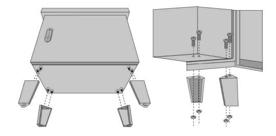
2. Place the backside of the cabinet on the ground and screw the 4 footholds
