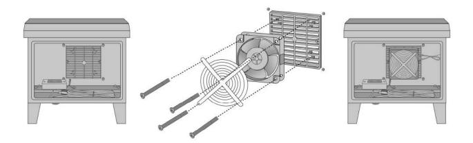
4. Fit the grill protector and the fan with 4 screws and fix them on the cabinet inner grill. The hump side should towards outside, if not do so, it would stuck the fan and buzzing when the power is on.
