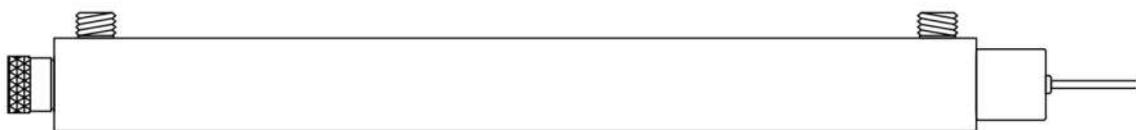
**STEP 6** Insert the whole UV bulb into the chamber, and cover a protective cap of the right side.
